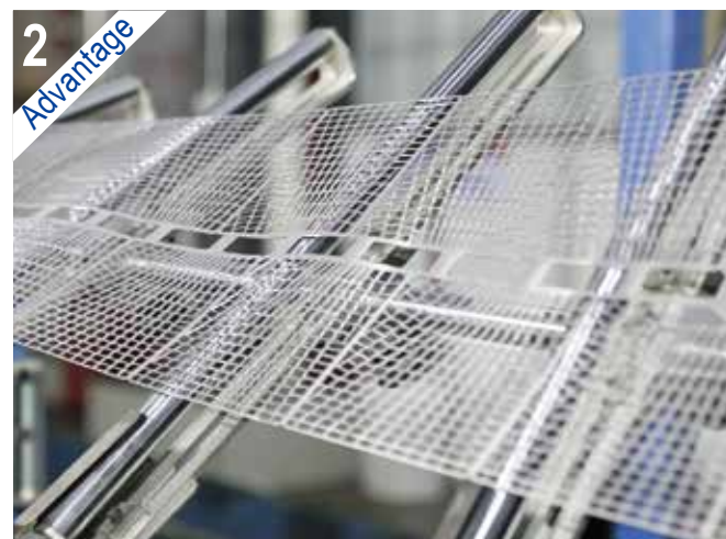
➤ Continuous casting and rolling grid The grid casted by the new continuous casting and rolling technology greatly reduces the corrosion of the grid, enhances the performance of the battery, and prolongs the battery life.
